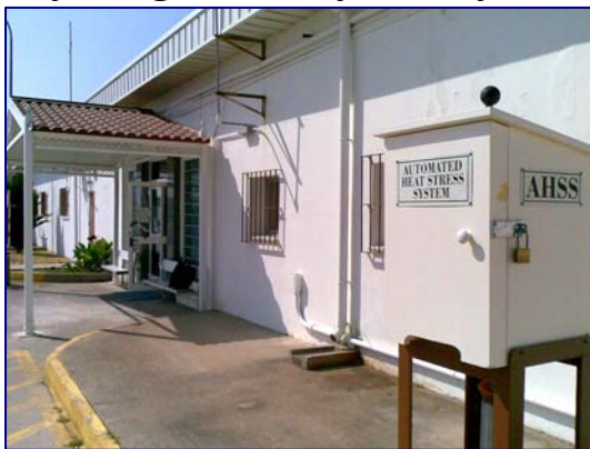
NAVSTA, Rota AHSS unit #2 deployed to the base Fitness Center for staff and patron awareness of ambient heat stress warning conditions in real-time.
