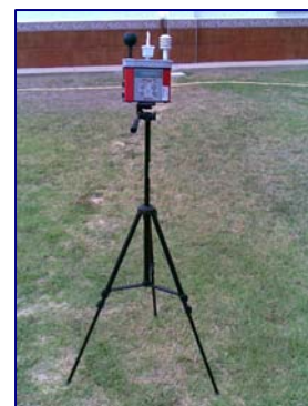
Traditional “wet wick” WBGT meters used by Rota’s IH Department were manually labor-intensive.
